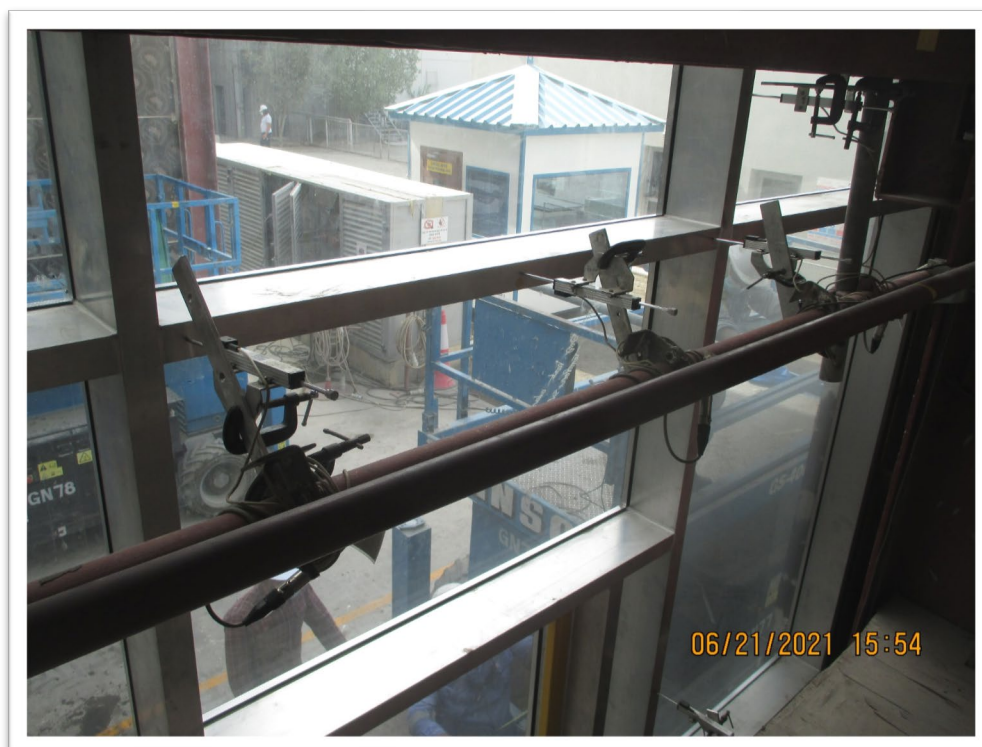
Arrangement of LDT's for Resistance to Wind Load Test – Serviceability & Safety
