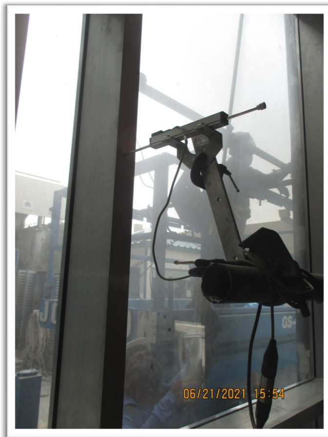
Arrangement of LDT's for Resistance to Wind Load Test – Serviceability & Safety
