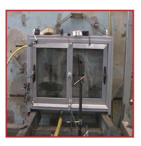
Watertightness & wind resistance test
